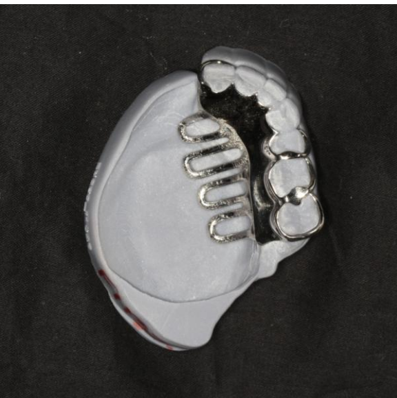
Fig. 4b – SLM printed framework on printed model
